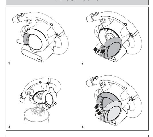
In order to keep the suction force optimised, the filters must be cleared regularly during use.
